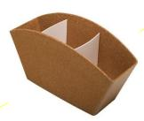
Injection moulded products with natural fiber reinforced polymer show good surface characteristics.
