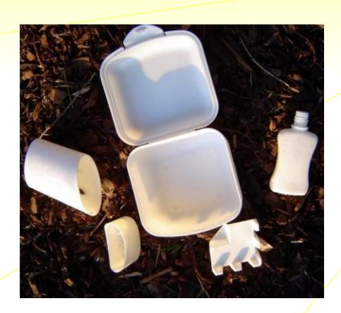
ARBOBLEND® is a mixture of different biopolymers like PHB, PLA, lignin, starch, natural resins and waxes, cellulose, Green-PE, Bio-PA and additives.
