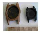
Injection moulding of ARBOFORM® with subsequent pyrolization results to pure carbon parts (99,9% concentration) with interesting electric conductivity properties and high dimensional stability under heat.
